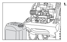
Place chemicals filter into container with additives
