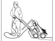
Never direct the high pressure jet at the high pressure cleaner itself! The high pressure cleaner may not be placed within reach of the high pressure jet spray mist!
