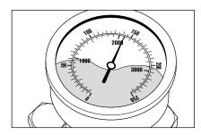
Having closed the trigger gun with safety catch, the high pressure cleaner must shut down and the stainless steel pressure gauge must show "O" bar. If not shut down and the stainless steel pressure gauge continuously shows full pressure gauge continuously shows full pressure, this could be due to leakage at the high pressure pump, at the pressure switch, at the high pressure hose or at the trigger gun with safety catch.
