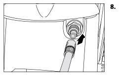
Connect water hose to water inlet (minimum requirements; 5 m hose length, cross-section <sup>3</sup>/<sub>4</sub>", 10 bar). The high pressure cleaner may be connected to a water mains (1-10 bar pre-pressure) with either cold or hot water (up to 60 °C). The medium quadro series provides the opportunity of sucking in water out of a container (see direct suction).
