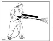
When using high pressure water for cleaning, make sure that there is a clearly noticeable recoil effect on the lance. Therefore ensure a firm footing (see technical data).
