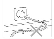
Only use a power supply cable in perfect working order! Do not damage or improperly repair the power cable (tearing, squeezing, running over, ...).
