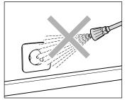
Never direct the high pressure jet at power sockets or any other electrical installations! Within the working area, all live parts are to be protected from both water jet and spray mist.
